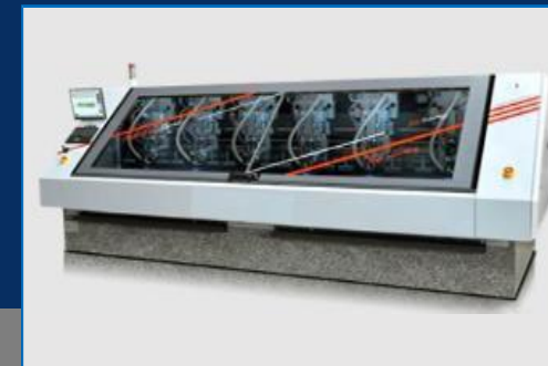
CCD mechanical drilling * (8)
