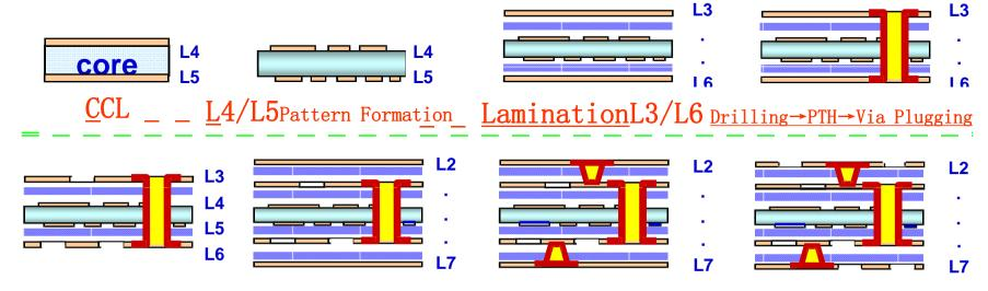
L3/L6 Pattern Formation Lamination L2/L7 Laser->Electroplating Pattern Formation L2/L7
