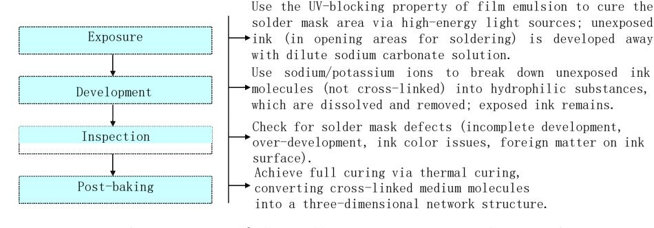
Note: Most inks cure at 150° C for 60 minutes. However, due to ink properties (e.g., thickness), immediate high-temperature curing may cause wrinkling (upper ink cures while lower ink does not). For viaplugged ink, direct high-temperature baking causes rapid bubble expansion and solvent evaporation (before full curing), leading to ink overflow from vias.
