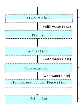
Remove surface oxides, roughen the board surface to ensure good adhesion between the subsequent electroless copper layer and base copper; the newly formed copper surface has strong activity for effective colloidal palladium adsorption. (Also protects the palladium tank from contamination by pre-treatment solutions, extending its service life.)
