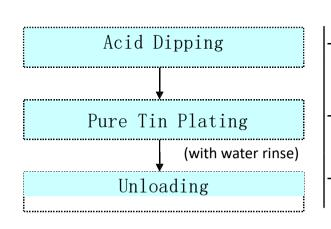
Remove surface oxides and activate the board surface; concentration is maintained at 8→ 10% to prevent water from diluting the sulfuric acid concentration in the tank.
